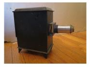
Projector, no light source. Hole in top to vent heat from candle or bulb. Slides are glass and each contain four colour images. Lens has two elements, one fixed at the back and the front element freely slides in and out of the lens-tube structure.
