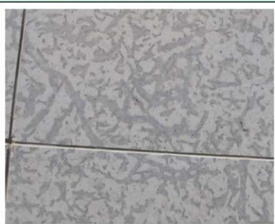
Mottled (burrowed) Tyndall Stone
