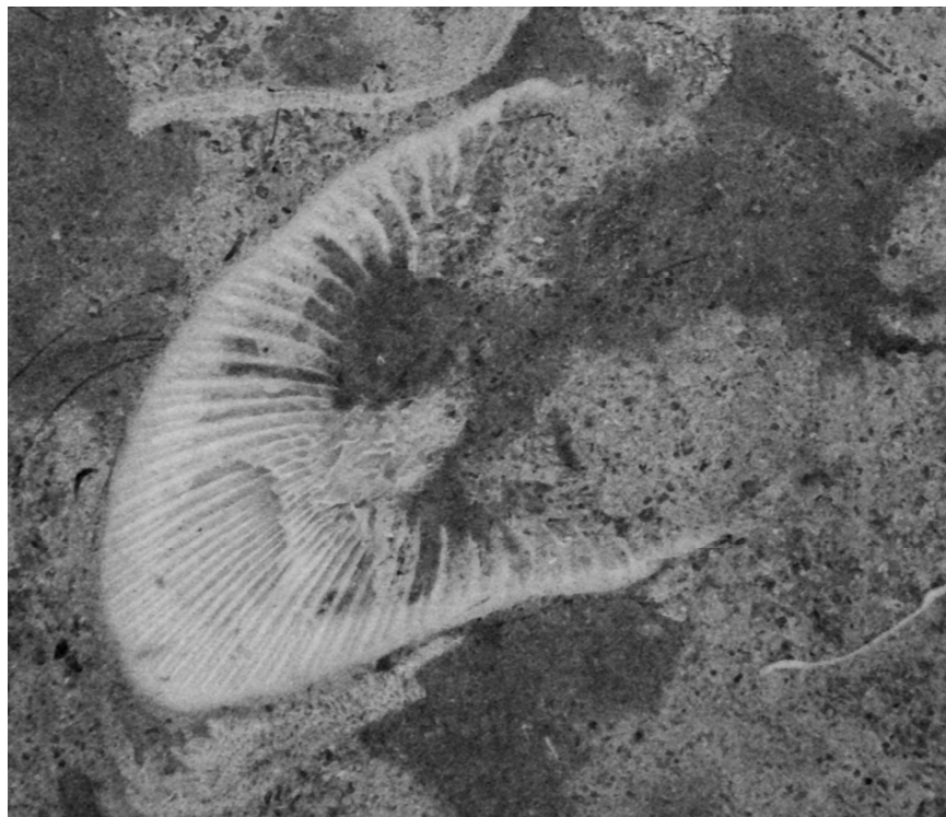
Figure 33: Cut section of Tyndall limestone with a section through a rugose coral showing the internal septa.
