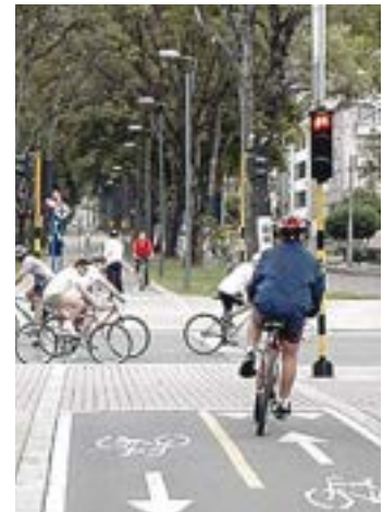
Figure C-64. Dedicated bike stop lights along bike routes.
