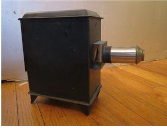
Projector, no light source. Hole in top to vent heat from candle or bulb. Slides are glass and each contain four colour images. Lens has two elements, one fixed at the back and the front element freely slides in and out of the lens-tube structure.
